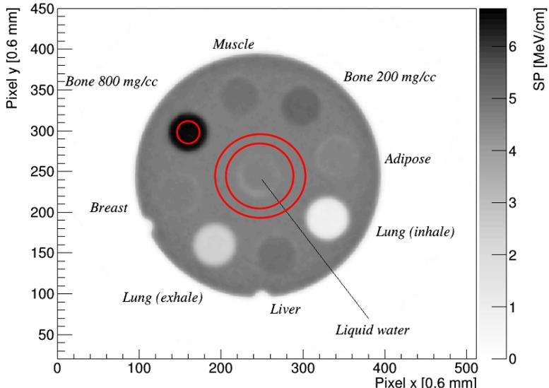
Distilled water vial used to normalize the Stopping Power values obtaining the Relative Stopping Power.
