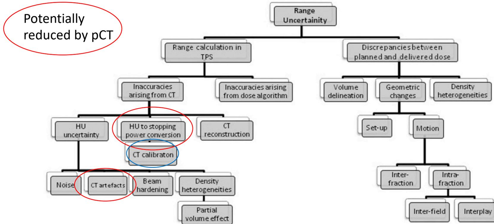
**Figure 2.** Schematic of sources of range uncertainties in proton radiotherapy. HU, Hounsfield unit; TPS, treatment planning system.
