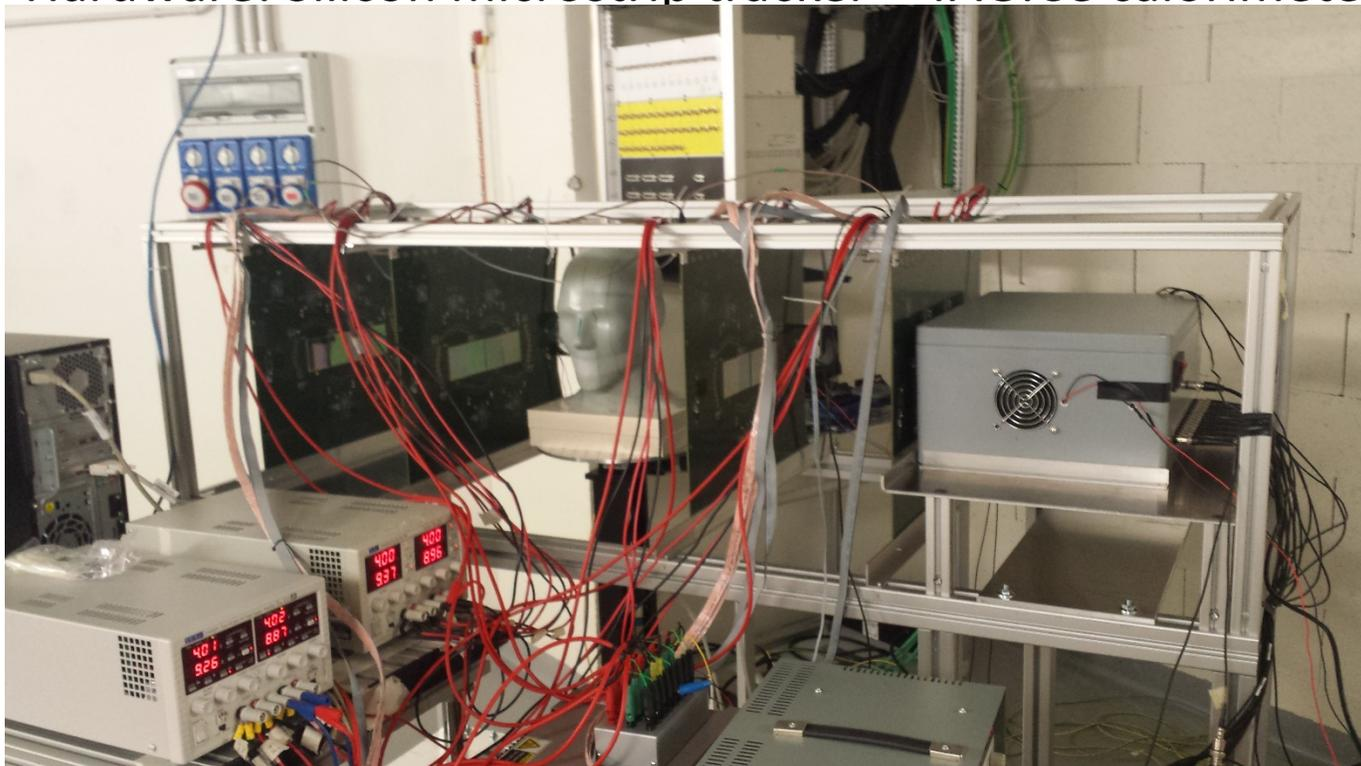
INFN pCT system under test with an anthropomorphic head phantom at Trento proton therapy center's experimental beam line
