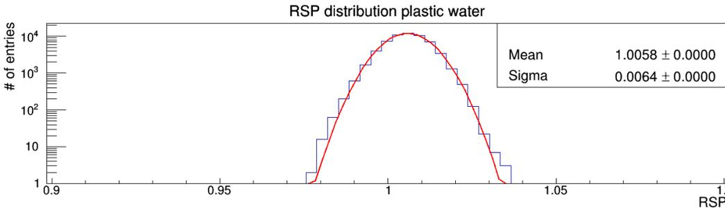
Measured RSP of the Plastic Water is 1.0058 (expected value 1.008)  $\sigma = 0.6\%$
