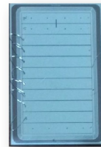
Type T 11 strips of 2.2 mm 2 (3993 μm x 550 μm) Pitch = 591 μm
