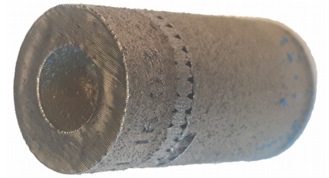
16 mm diameter 3D printed nickel
